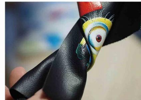
Stretch test for UV soft ink
